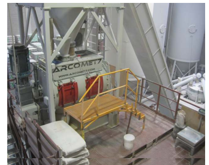
HLV-1500 2C / Dry mortar Plant
