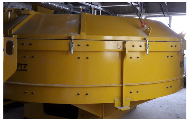
Mixer used for glass processing.
