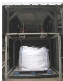
Big bag filling by weighing platform.
