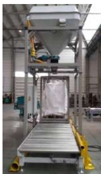
Automatic big bag filling system with roller path, carousel.
