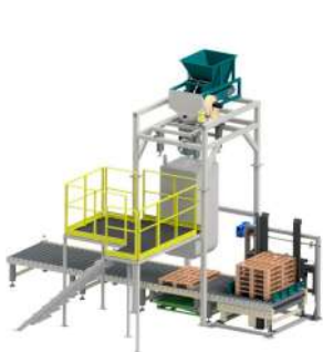
Automatic big bag filling system with roller path, carousel.
