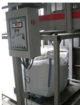
Big bag filling by weighing platform.
