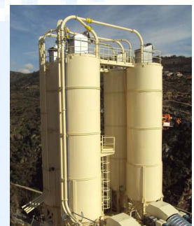
Pneumatic transport for cement and ash to different destinations. Continuous supply to plant.
