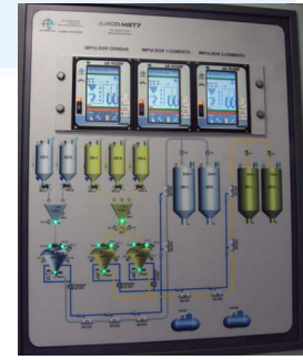
Automatism to control mixing process and pneumatic transport in dense phase. Finished product is loaded in a silo.
