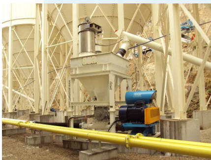
Dilute phase pneumatic transport.
