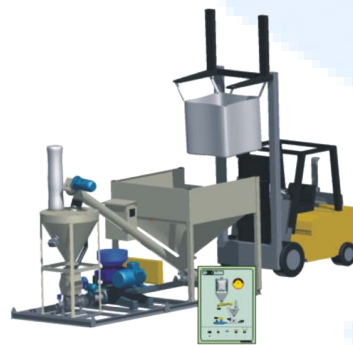
Mobile pneumatic conveyor for big bag discharge
