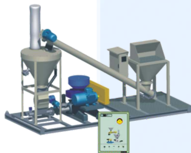
Mobile pneumatic conveyor for bag opening
