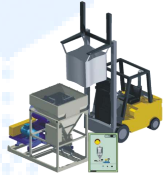
Mobile pneumatic conveyor for big bag discharge
