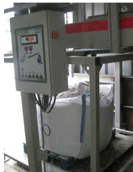
Big bag filling by weighing platform.
