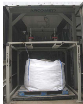
Big bag filling by weighing platform.
